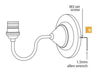
Place the fixture canopy onto the backplate. Level the fixture vertically and tighten the two M3 set screws with the 1.5mm allen wrench to secure the fixture in place.
